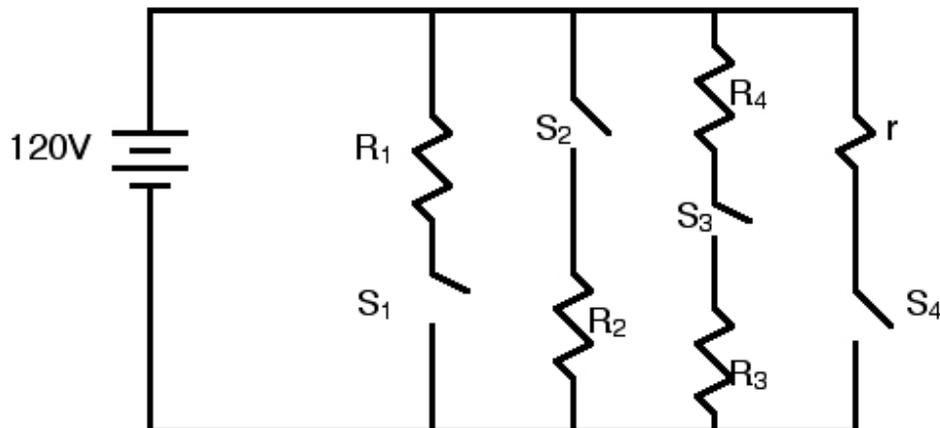
Switches  $S_1$ ,  $S_2$ ,  $S_3$ , and  $S_4$  can be open (no current will flow) or closed (current flows through the switch freely). Resistors  $R_1$  and  $R_3$  are the 60 watt bulbs,  $R_2$  is the 1500 watt hairdryer and  $R_4$  is the 100 watt light bulb. Switch  $S_4$  is open for now. The resistor  $r$  is  $1 \Omega$ . It represents a possible short-circuit that develops if switch  $S_4$  is closed.
